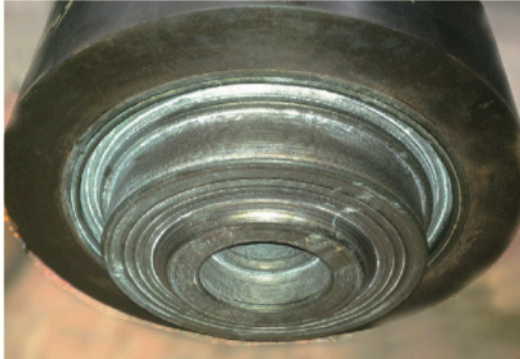
Inconel 625 Alloy etc. Welding Overlay (Min. 3mm)
